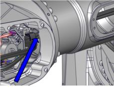
Remove the cable harness out of the arm tube, at the back of the upper arm.
