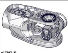
If axis 5 is not already in position +90°, connect the brake release tool, release the User instructions are enclosed with the brakes and move the axis manually into that position.
