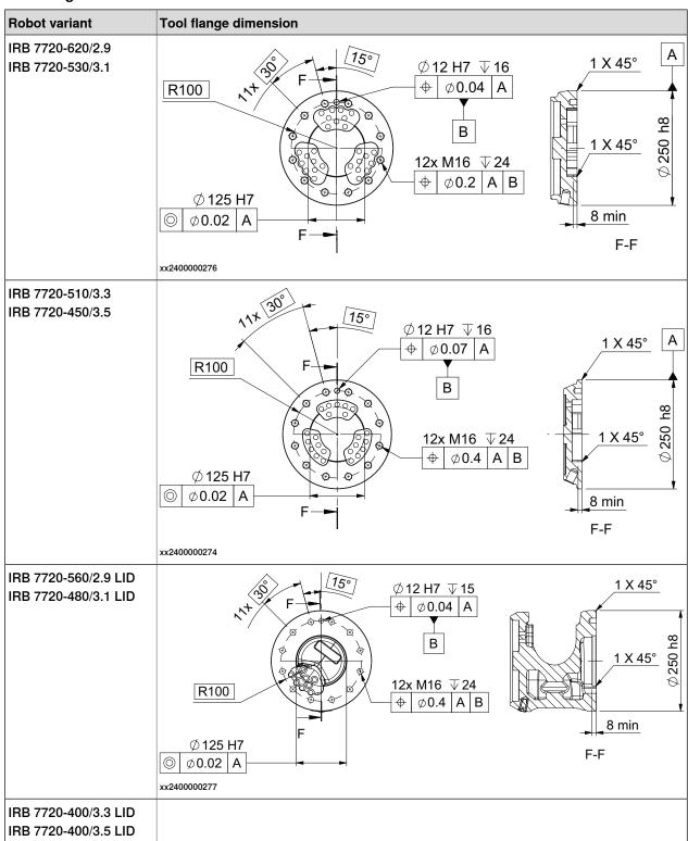
3.3.7 Fitting equipment on the robot (robot dimensions)
